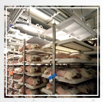
**PRE-REST:** after the salting phase, the ham is washed, dried and placed in the pre-rest cells. In the latter, working with very low humidity and temperature, dehydration is obtained and salt is helped to work, which will penetrate evenly inside, towards the center of the ham
