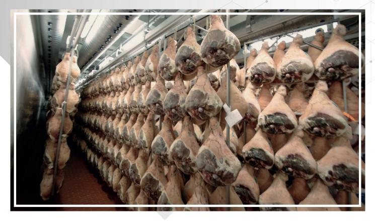
**DRYING:** during this phase (the duration of which depends on the weight of the ham) the temperatures begin to rise to encourage the initiation of the ripening process
