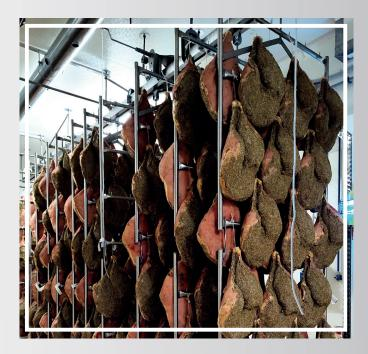
**SEASONING:** is the final stage of the process. With appropriate technologies, the control of temperature and humidity is guaranteed and the correct re-oxygenation of the environments is given. Constant parameters and air exchange are essential to develop, during the cycle, the flavor of the ham
